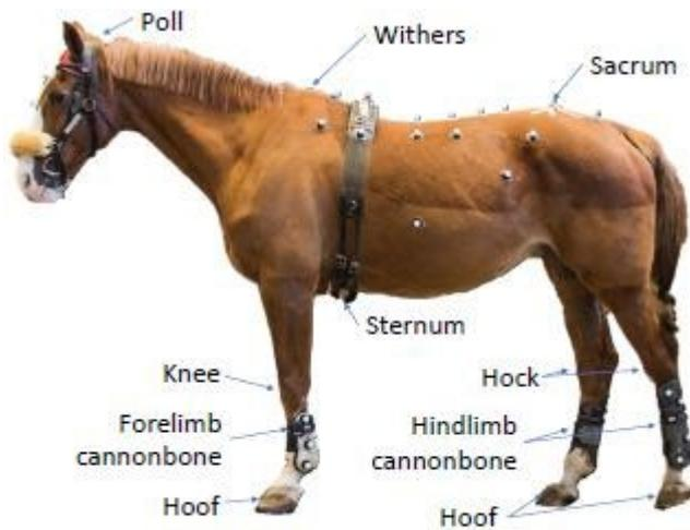
Figure 2. Photographical illustration of a horse equipped for a multi-sensor based gait analysis system (EquiMoves®).
